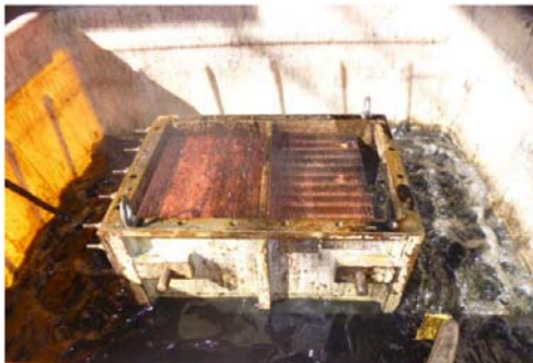
Submerged Cleaning in CREPEARL Solution (Circulated by compressed air/implemented by halves in 2 times)
