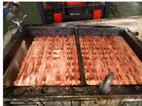
Air Cooler Core after Cleaning (Submerged in 10% solution of KURIPPEARL S320 for 5 hrs.)
